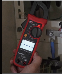
NCV multi-segment display and audio/visual alarm
